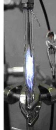
Fig.3. Reactor's non thermal plasma discharge
