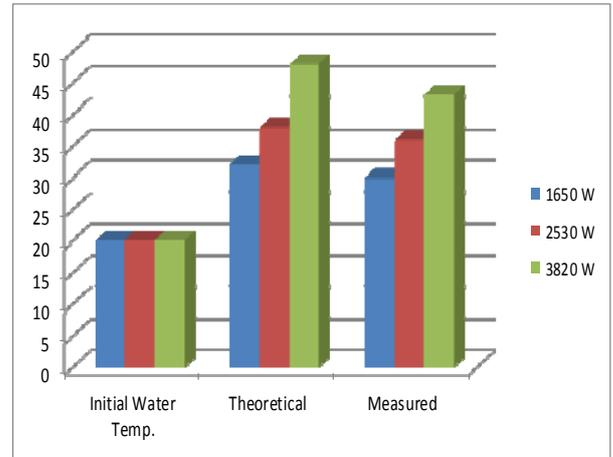
Fig. 5. Temperature values vs. consumed power
