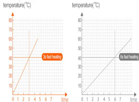
Fig. 2. Evolution of temperature vs. time in the case of existing and proposed heating system
