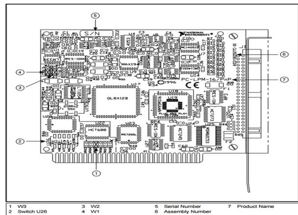
Fig. 3. Data acquisition board - main components
