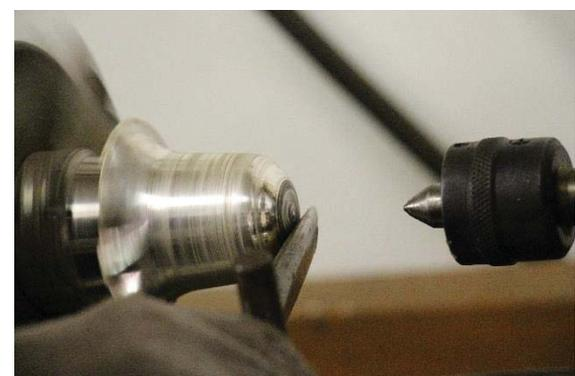
*Fig.4. Subsequent steps of preparing metal spinning cup.*
