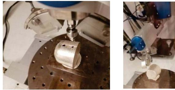
Fig.6. Pole figures measurement of a) metal spinning and b) wrinkling cup by centreless X ray diffractometer.
