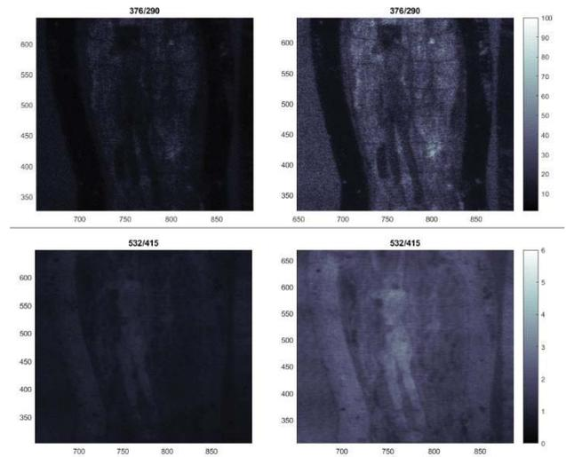
Fig. 7. Application of calibration ratios to FORLAB fluorescence ratios 376/290 and 532/415. Left: without calibration. Right: with calibration
