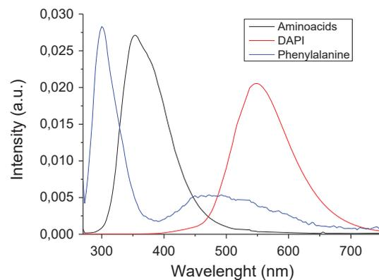
Fig. 1. Fluorescence spectra of the reference solutions.
