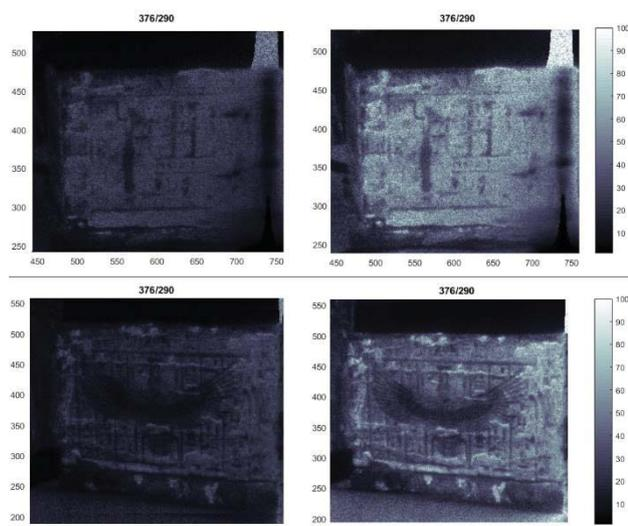
Fig. 8. Application of calibration ratios to FORLAB fluorescence ratio 376/290 of casket sides. Left: without calibration. Right: with calibration
