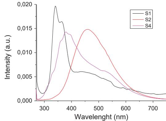
Fig. 3. Fluorescence spectra of sections S1, S2 and S4 of marble tile.
