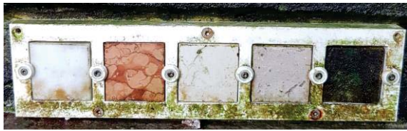
Fig. 2. Samples in position 1 placed at Palazzo Malipiero (Venice) after six months of exposure. From left: marmo di Carrara; rosso di Verona; pietra d'Istria, pietra di Aurisina and pietra di Vicenza. The latter is completely covered by an organic patina.
