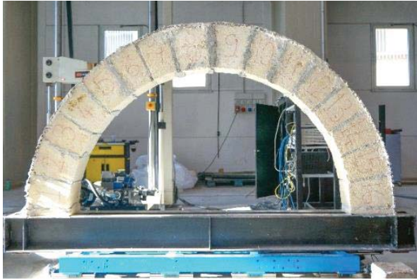
Fig. 2. GFRCM reinforced arch
