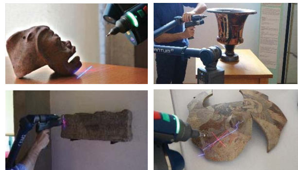
Fig. 4. Measurement through the 3D laser-scanner arm
