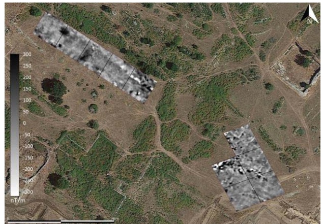
Fig. 4: Gradiometric contour map of the investigated area. Range -300 – +300 nT/m
