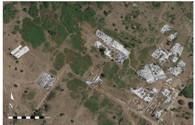
Fig. 3. GPR time slices at the estimated depth of 1.20 m.
