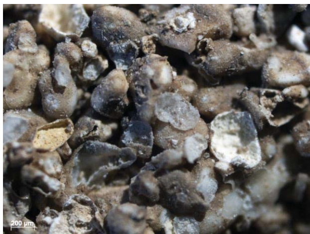
Fig. 3. Sandstone under reflected light microscopy
