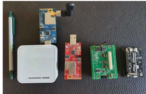
Fig. 2. Motes used for IoT-MHECHA (from left to right): CM5000 (connected to the gateway), XM1000, IRIS (with MDA300CA), LoPy4 (on top of PySense).
