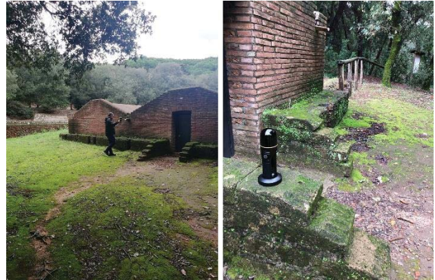
Fig.2: Leica personnel scanning the "Area delle Cisterne" and the Leica BLK2GO with its base.
