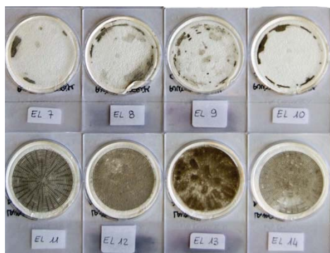
Fig. 6. Quartz fibre filters where DMP has been collected by the different cleaning procedures.
