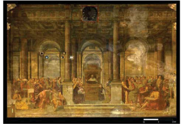
Fig. 7: Orthophoto of the fresco (original nominal scale 1:50, pixel resolution of 2 mm).
