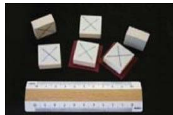
Fig. 2: Targets employed to create an ad-hoc grid for the calibration of the thermal camera and during the survey of the fresco
