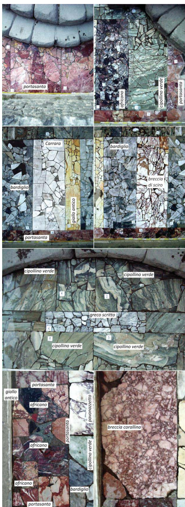
Fig. 5. Detail of some of the main varieties of ancient stones and marbles present in the reconstituted opus sectile of the Odeion.
