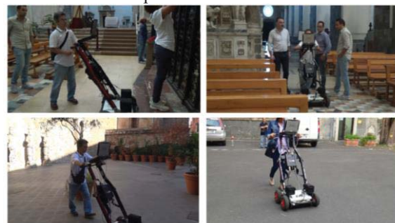
Fig. 2. The phases of GPR data acquisition
