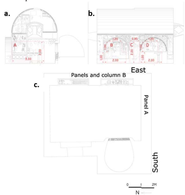
Fig. 4. Schematic map of the frescoed walls investigated in the Crypt: a) the panel A investigated on the south wall; b) the masonry elements (panels B and D, column C) investigated on the east wall; c) the plan of the Crypt with indication of the investigated areas.
