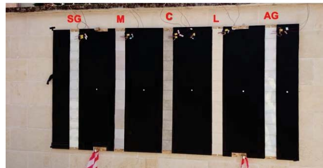
Fig. 2. Panel with material (zoom of figure 1e). SG: Standard Glass; M: Marble; C: Ceramic; L: Leccese stone; AG: Autocleaning Glass.
