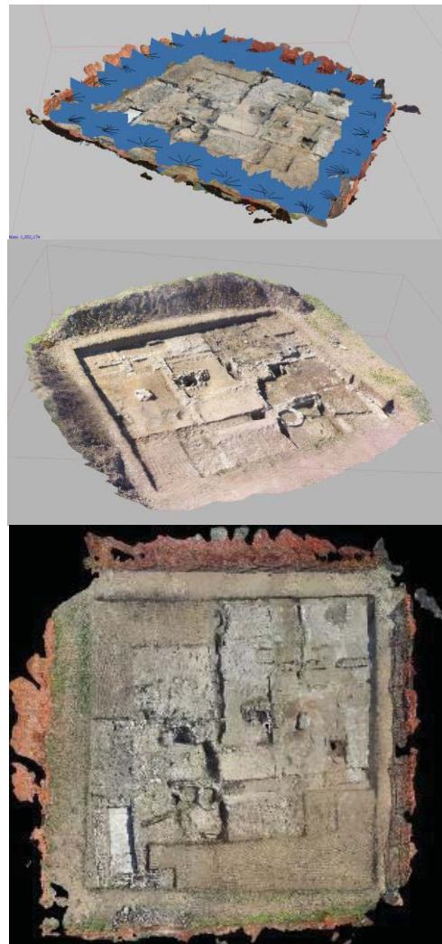
Fig. 1 – Top: 3D-Model of the Archeological excavation in Luni (2017-Photos by J.Lucchesi, smartphone). Middle: 3D-Model taken by a drone; Bottom: Orthophoto of the site, from the model obtained on the ground with the smartphone.
