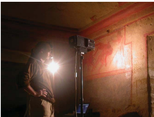
Fig. 4 –Hyperspectral acquisition of a mural painting in a Etruscan Tomb (Tomb of the Monkey, V century b.C.)
