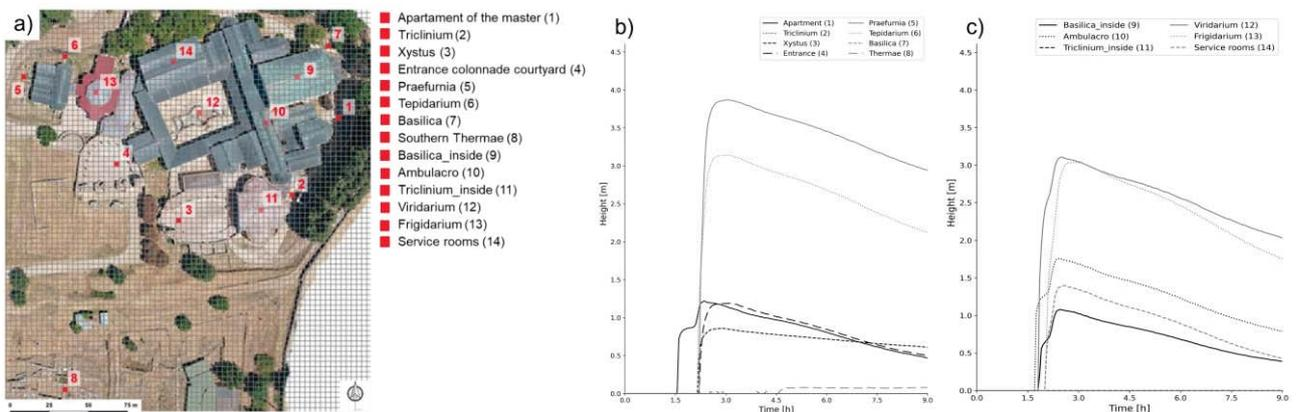
Figure 3: (a) position of the control cells, inside and outside of the archaeological area for "open Villa" model (b) trend of the heights of the debris flow for one of the simulations in outside control cells (c) trend of the heights of the debris flow for one of the simulations in inside control cells.
