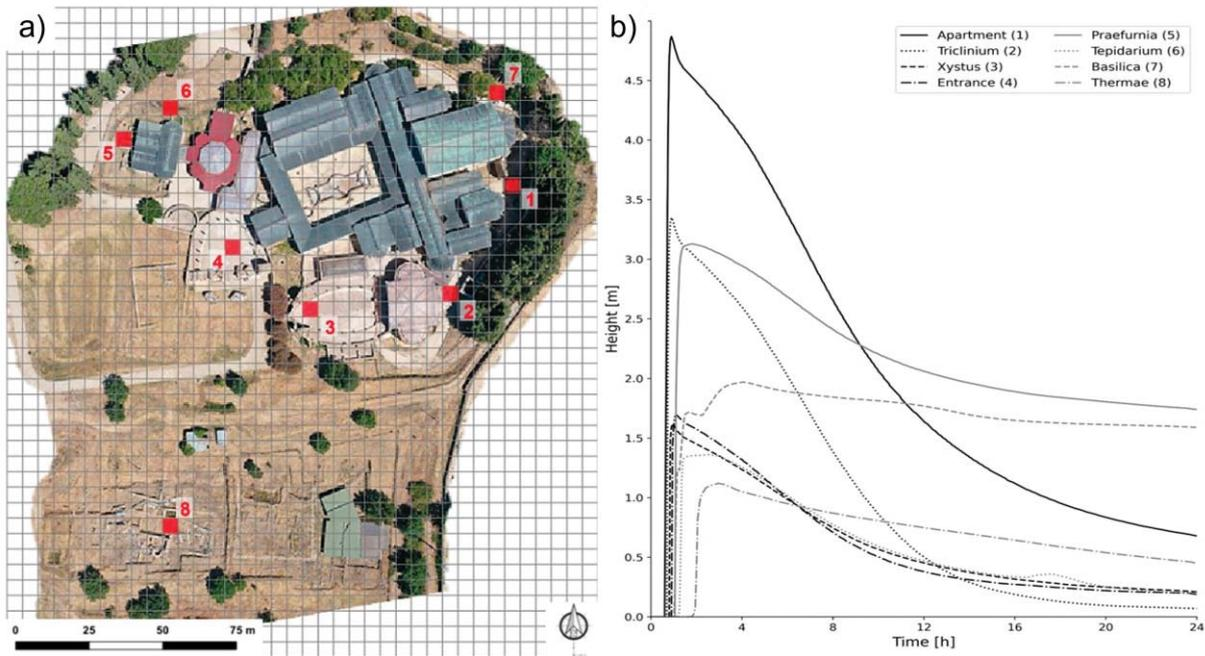
Figure 2: (a) position of the control cells within the archaeological area for "closed Villa" model (b) trend of the heights of the debris flow for one of the simulations.
