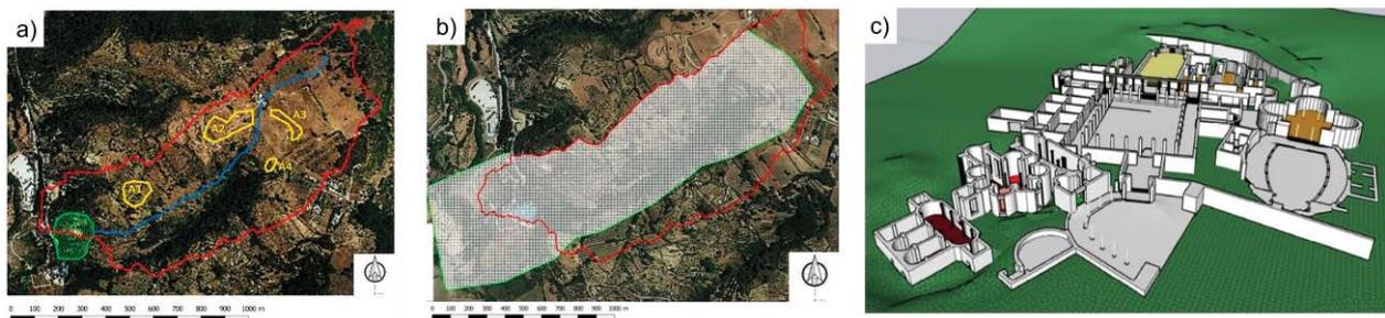
Figure 1: (a) Identification of the 4 unstable area (b) numerical model with 5x5 meters square mesh grid (c) 3D model of the Villa Romana del Casale
