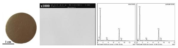
Figure 2. Photograph, SEM image and EDS spectra of bare CNR- alloy. The EDS spectrum on the left was recorded on a large area and the one on the right on the white islands.
