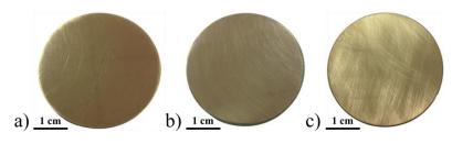
Fig. 3. Photographs of alloy disks with different surface roughness: a) 555-SF1, b) 555-SF2 and c) 555-SF3.
