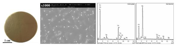
Figure 1. Photograph, SEM image and EDS spectra of bare 555 alloy. The EDS spectrum on the left was recorded on a large area and the one on the right on the white islands.
