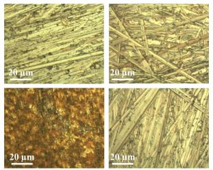
**Fig. 4.** Micrographs of the quaternary 555 alloy disks with a high roughness before (first row) and after (second row) corrosion treatments with HCl/H2O vapours for bare alloy (on the left) and coated with chitosan-BTA (on the right).
