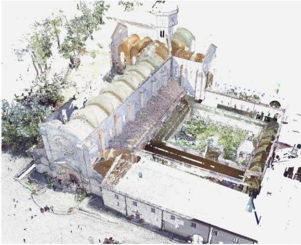
Fig. 1. Point cloud created by laser scanner of the abbey complex of Fossanova.
