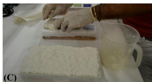
Fig. 3. (A) One of the mock-ups at the end of the preparation; (B) application of NanoRestore®, and (C) application of DAP.
