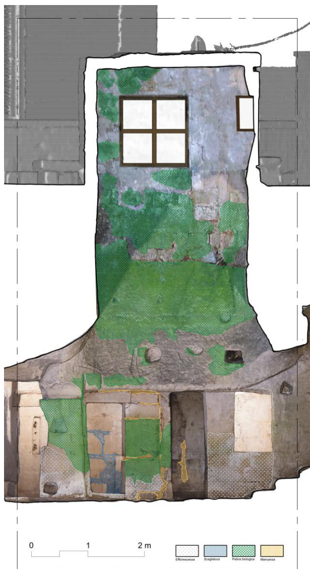
Fig. 8. Hypogeum oil mill of Melpignano: surface degradation mapping.
