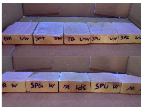
Fig. 4. Different application methods on limestones. W=wet samples, on air application; UW=underwater application; BR=brush, SPT=spatula, TB=toothbrush, SPU=PVA sponge, SPG=sponge.
