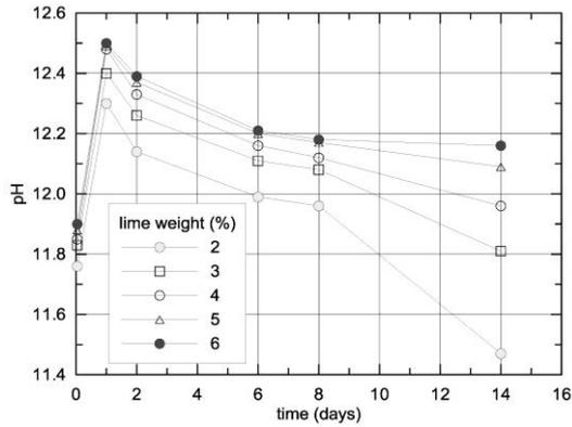
Fig. 2 - Evolution of pH for pozzolana-lime-water solutions over 14 days.
