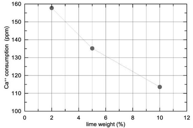
Fig. 3 -  $Ca^{2+}$  consumption after one hour curing for different lime percentages
