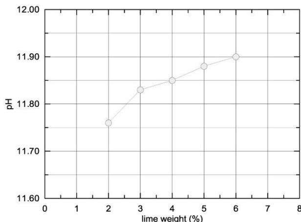
Fig. 1 - Value of pH for pozzolana-lime-water solutions after one hour curing.
