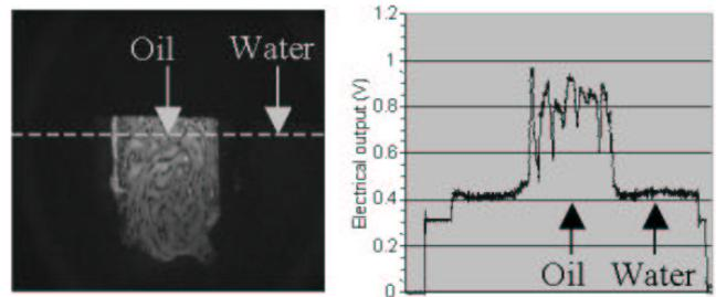
Fig. 7. Very low diesel oil thickness detection with “black light”
