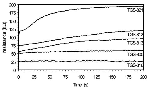
Fig. 1. Time evolution of Figaro TGS sensors' electrical resistance when exposed to a 1ml oil sample
