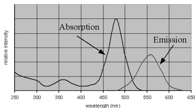
Fig. 2. Emission and absorption (excitation) spectra of a typical fluorochrome
