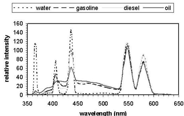
Fig. 5. Fluorescence spectrum measured with the PMQII on various pollutants and wastewater
