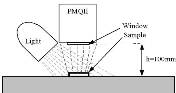
Fig. 4. Configuration of the spectrofluorometer
