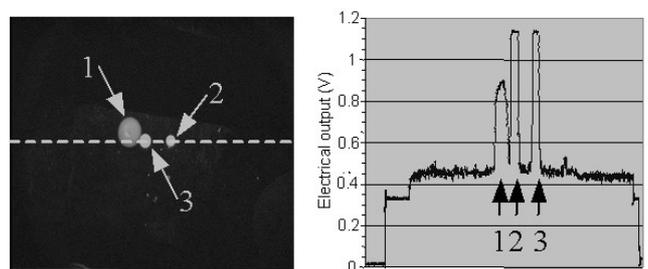
Fig. 8. Detection of various hydrocarbons with black light (1 : heating oil, 2 : oil type 2, 3 : gasoline)
