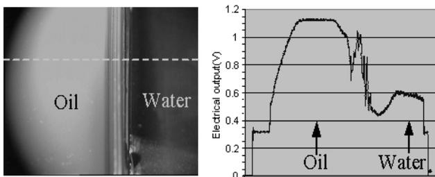
Fig. 6. Contrast obtained with the detection system between oil and water (CCD camera frame on the left ; electrical signal of one line - shown by a dotted line on the frame - on the right)
