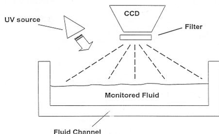
Fig. 9. Configuration of the in situ detection system
