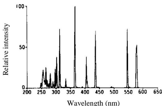
Fig. 3. High pressure mercury spectrum
