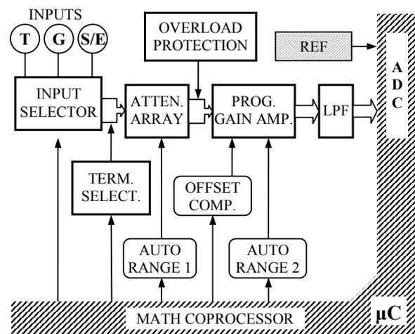
Fig. 4: A detailed analogue section overview
