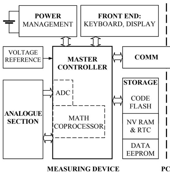
Fig. 3: Measuring device hardware structure
