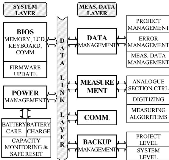
Fig. 5: Measuring device firmware structure – layered event driven conception
