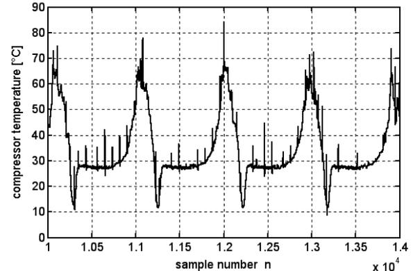
Fig.6. Fragment of exemplary registered signal of temperature changes in compressor - signal 6 (total samples number is equal 600 000)
