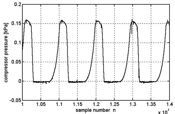
Fig.7. Fragment of exemplary registered signal of pressure changes in compressor - signal 7 (total samples number is equal 600 000)
