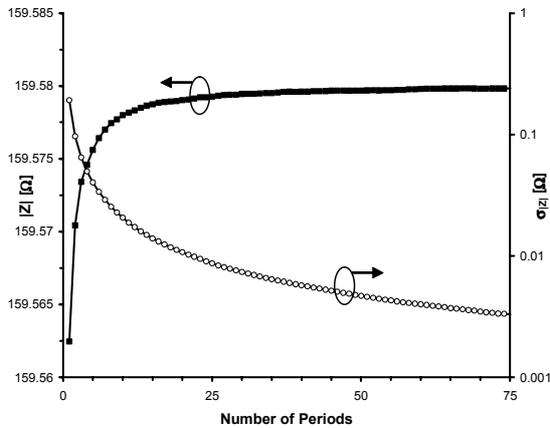
Fig. 5. Average value of the modulus of the impedance and the respective standard deviation. The results correspond to 1000 tests performed at 1kHz with 24390S/s using  $\bar{Z}_{R1}$  as the sampling impedance.
