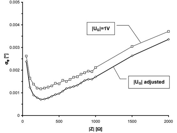
Fig. 3. Standard deviation of the measured phase obtained with a 12 bit digitizer and a sampling rate of 24390S/s. The input frequency is 1kHz and 1000 records of 976 samples corresponding to 40 periods were acquired and processed.
