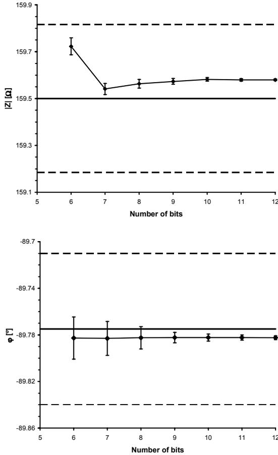
Fig. 7. Measurement results of  $\bar{Z}_1$  and respective standard deviations ( $2\sigma$ ) as a function of the ADC resolution (164 periods and 24390S/s at 1kHz). The solid thicker lines correspond to the value determined by the HP4192A and the dashed lines represent the interval limits due to the error of the HP4192A.
