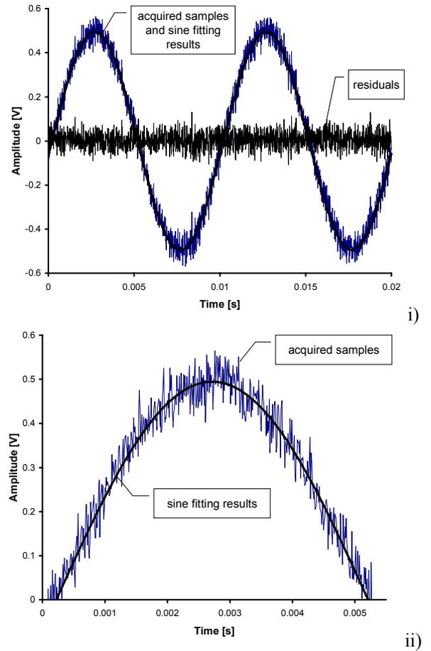
Fig. 2. Sine fitting results in a very noisy environment. In i) the acquired samples and the results of the fitting overlap while the residuals show the added noise. ii) corresponds to a zoom in the section of the first maximum.
