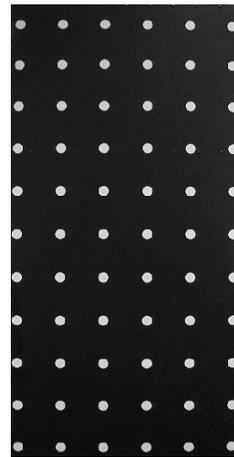
Fig. 1. Black calibration plane with  $6 \times 11$  white circled markers painted on
