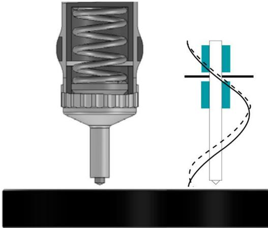
**Figure 2: UCI schematic principle**
