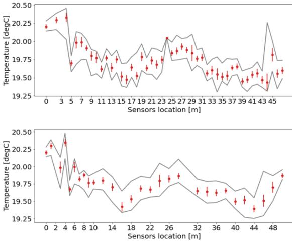
Fig. 3: Temperature profile in space for test case 5 simulating a real measurement for the two repetitions A (top) and B (bottom). The circular marker is at the mean value and the error bars are at plus minus one standard deviation. The lines above and below connect the maximum and minimum measured values during the entire time span.
