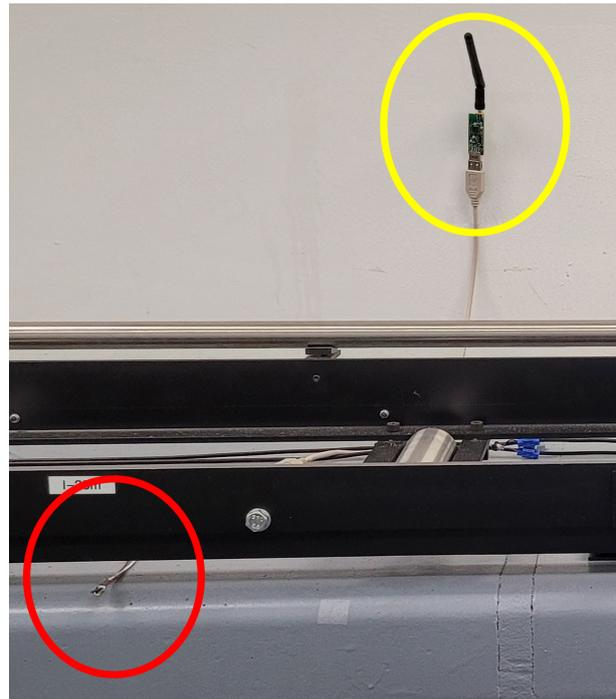
Fig. 1: The horizontal black parts are the rails for the cart used in the interferometer set-up. In the red circle at the lower left corner a the sensing part of a temperature sensor node is visible. In the yellow circle in the top right corner a router node with external antenna is visible, connected to the wire supplying power by means of a USB connector.
