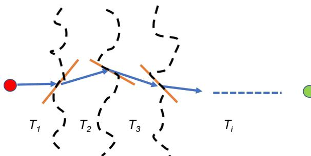
Fig. 2: Two dimensional simulation of curved light paths due to refraction effects. The vertical curvy black dashed lines delimit zones with different temperatures. The slanted orange lines indicate the assumed direction of the local interface between these zones. The light is assumed to travel from the red spot on the left to the green spot on the right and back.
