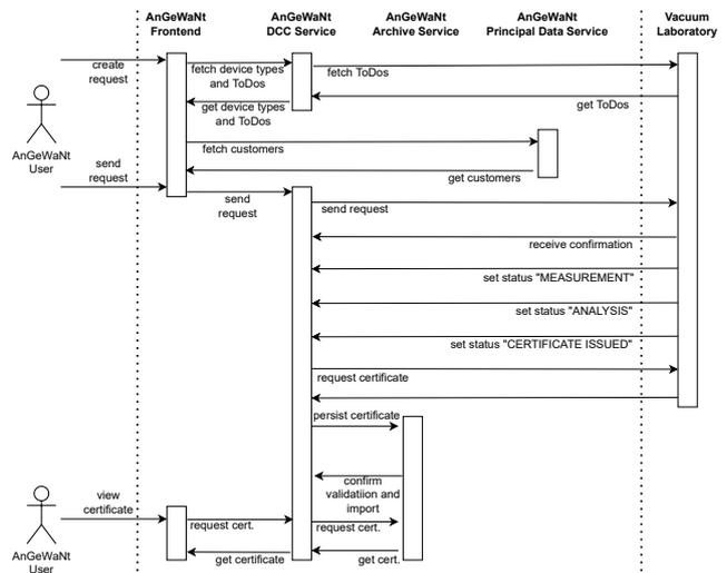
Fig. 2: Sequence diagram of the interface integration to enable communication between Vacuum Metrology Group, and the AnGeWaNt platform.
