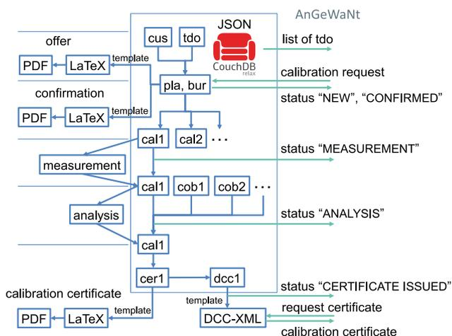
Fig. 3: Workflow of calibration application in the Vacuum Metrology Group, and its integration with AnGeWaNt by sending status codes via PUT to the specified REST endpoint of AnGeWaNt's DCC service.
