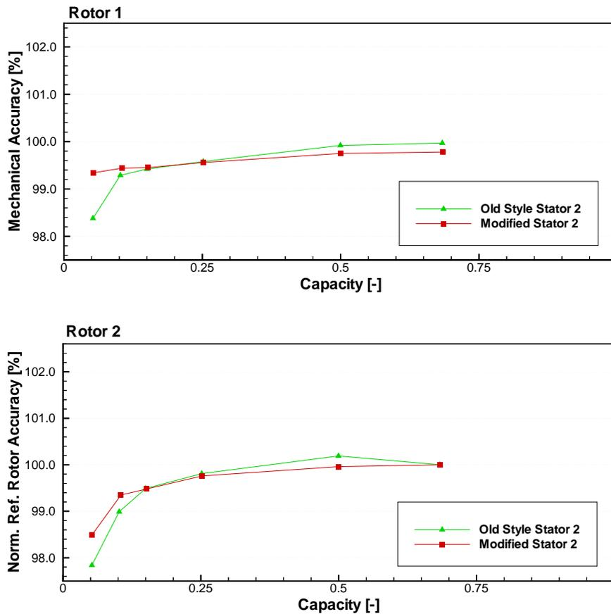
**Figure 7.** Comparison of accuracy curves for the original and the modified design of the second stator at a pressure of 27 *psi*.
