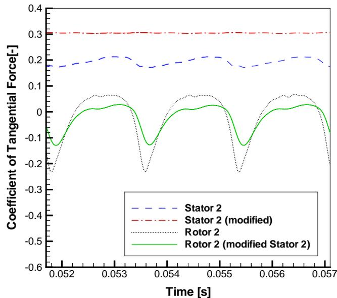
**Figure 6.** Comparison of coefficient of tangential force of reference stator (2) and reference rotor (2) for the original and the modified design with a shortened reference stator (2).
