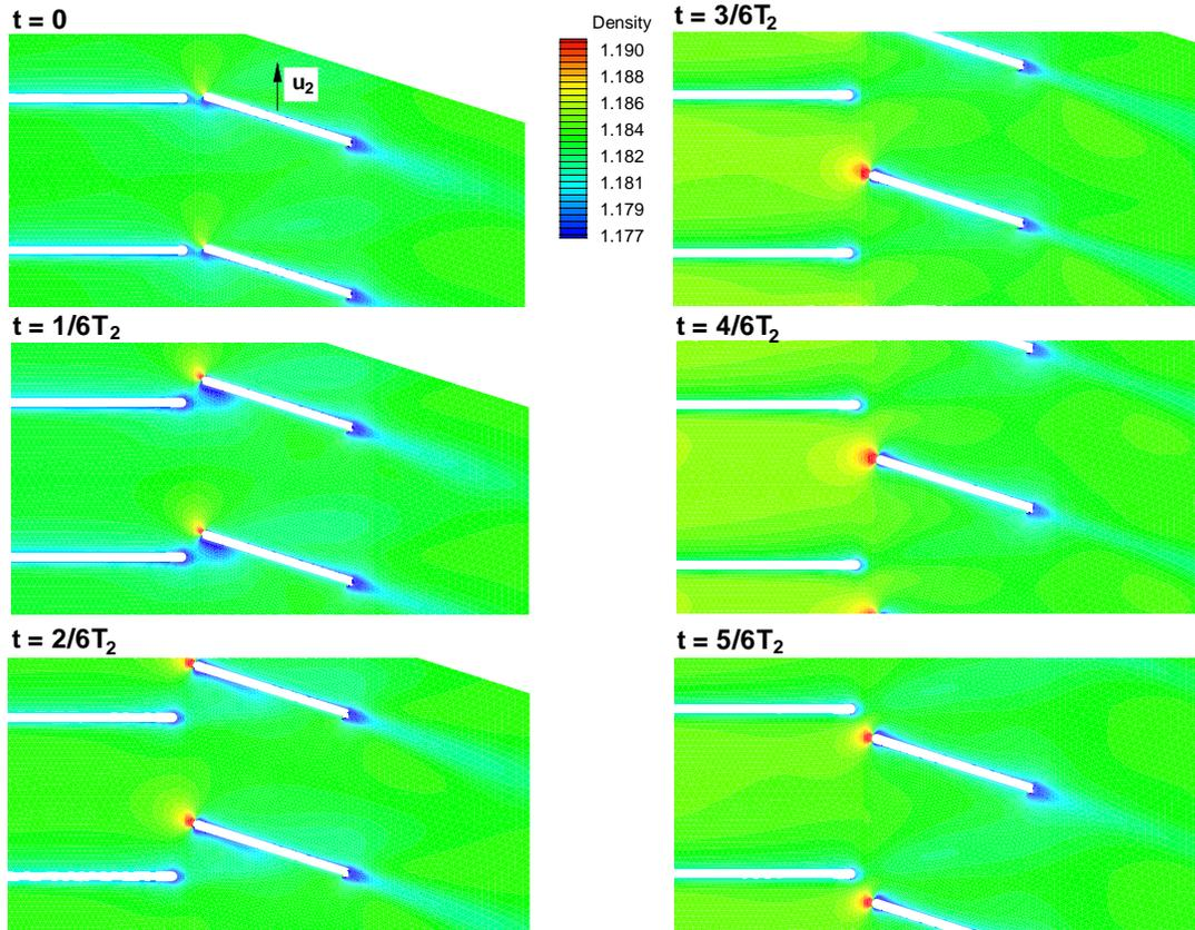
**Figure 4.** Density contours for one period of the second stage of the turbine flow meter.
