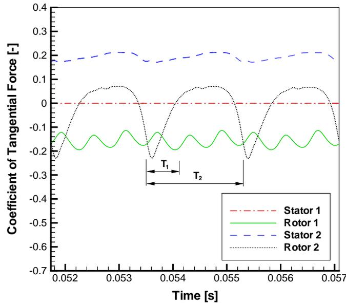
**Figure 5.** Coefficient of tangential force versus time for both stators and rotors for a periodic state.
