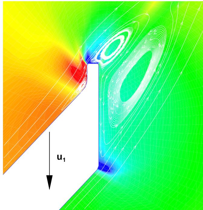
**Figure 3.** Pressure contours and streamlines of relative velocity at the trailing edge of the first rotor.
