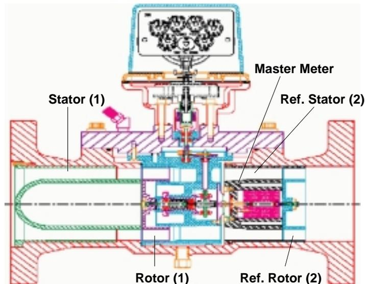
**Figure 1.** Cutaway drawing of the two-stage AccuTest<sup>TM</sup> turbine flow meter.
