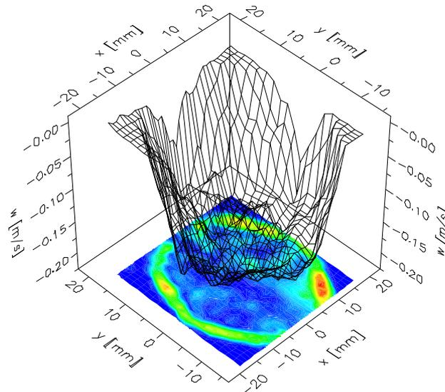
**Figure 7** Instantaneous three-dimensional velocity field along the pipe cross-plane: meshed geometry represents out-of-plane velocity component magnitude; color-flooded contour shows in-plane velocity magnitude distribution.
