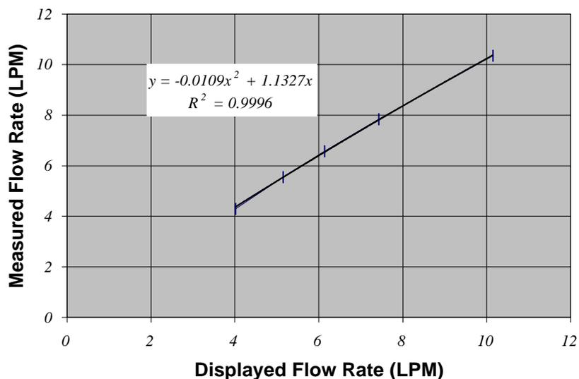
**Figure 6** Flow meter calibration using volume-over-time method.
