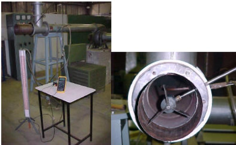
Figure 11 - Assembly of the prototype and of the Plandtl tube in the work-bench
