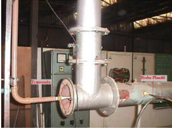
**Figure 8** - Assembly of the probes in the pressure tube of a fan
