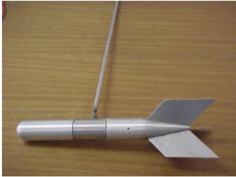
Figure 10 - Prototype of the transonda.
