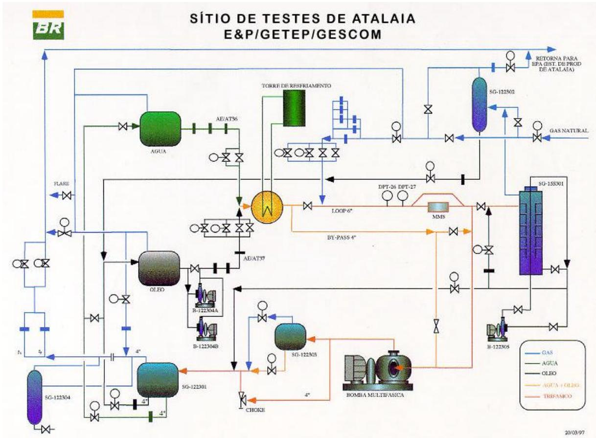
Figure 01- Flow Diagram: Atalaia Multiphase Flow Test Facility
