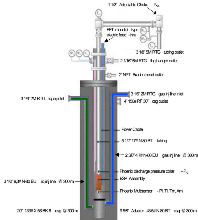
**Figure 03.** Well Test Facility
