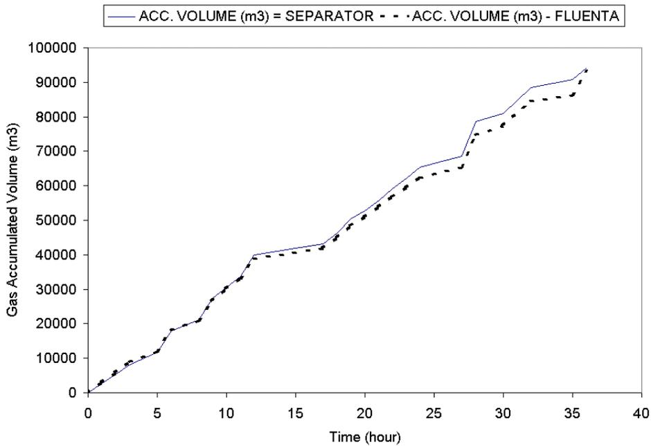
Figure 7.4 Accumulated gas volume versus time, measured by the Fluenta meter and the test separator.
