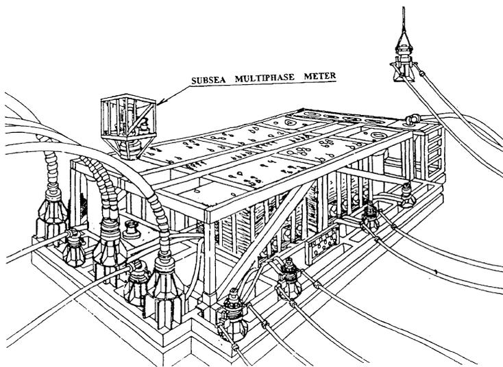
Figure 6.2 The subsea production manifold MSPDL-3, with retrievable multiphase meter module.
