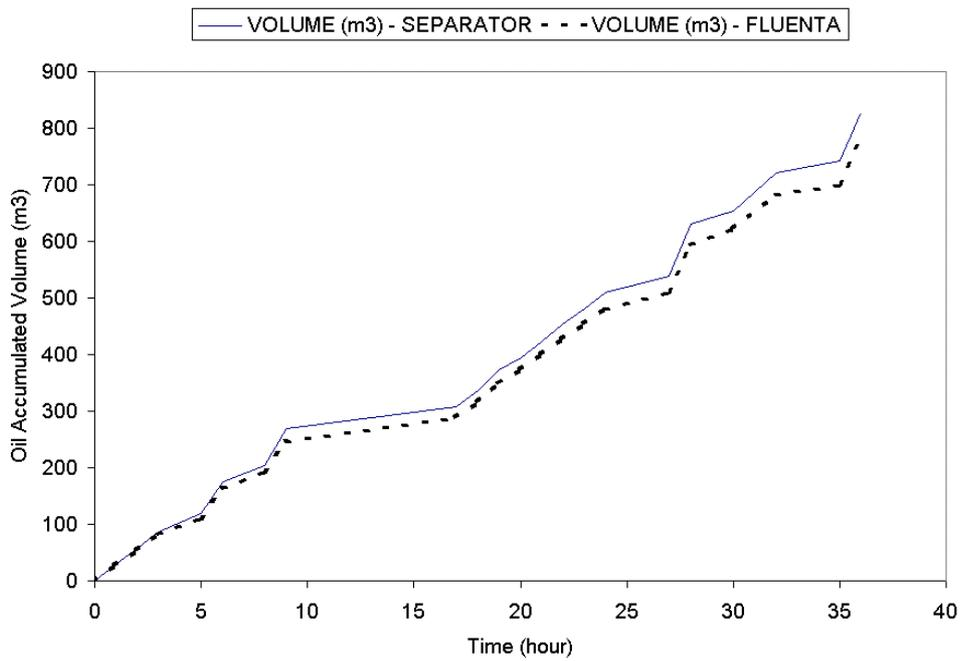
Figure 7.2 Accumulated oil volume versus time, measured by the Fluenta meter and the test separator.
