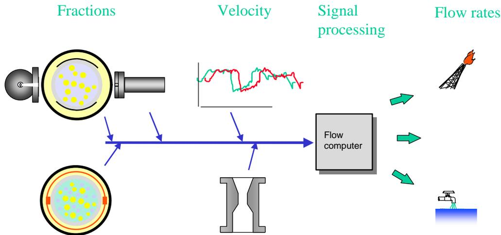
Figure 4.2 The Fluenta MPFM 1900VI; Measurement principle
