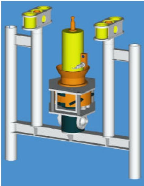
For future applications of subsea multiphase metering, Fluenta has developed a new generation compact ROV retrievable version: The MPFM 2000 SR system design is based on the topside meter, MPFM 1900 VI and the previous Fluenta subsea flowmeter, the SMFM 1000. The basic elements are the same as for the previous subsea meters, with a number of improvements and re-packaging.
