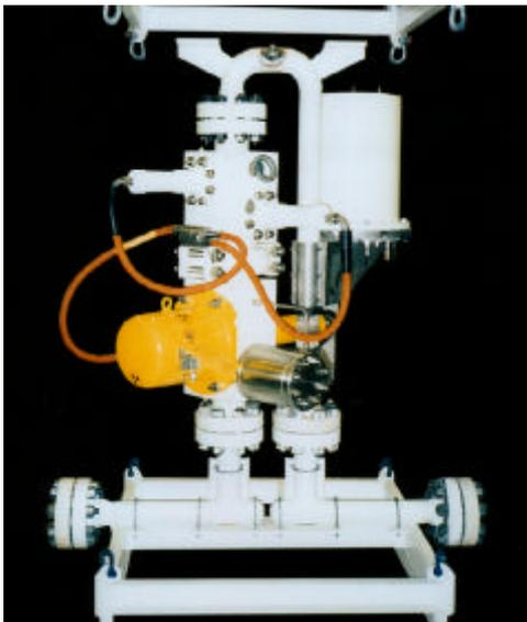
Figure 5.1 The Fluenta SMFM 1000, mounted on test skid.
