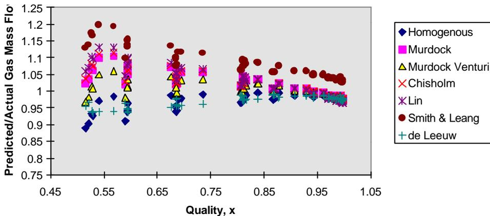
Figure 2. Comparison of all seven correlations using 40 bar data.
