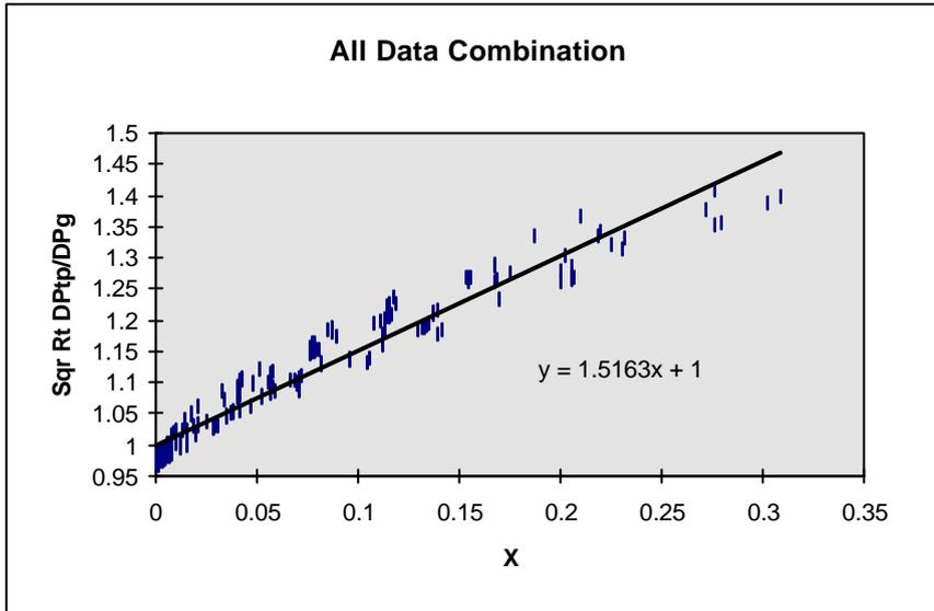
Figure 4. A Murdock Type Graph with Venturi Data
