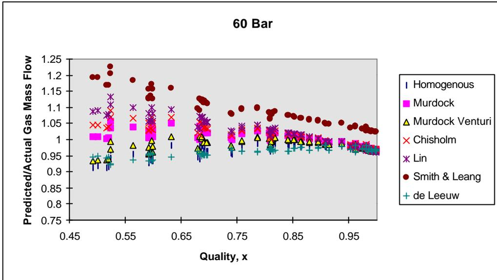
Figure 3. Comparison of all seven correlations using 60 bar data.
