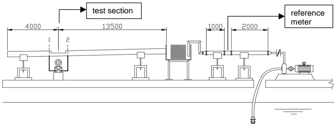
The reference meter, an electromagnetic flow meter for running full pipes, was calibrated in a Laboratory accredited by PTB – Physikalisch Technische Bundesanstalt. The uncertainty is  $\pm 0,31\%$ .
