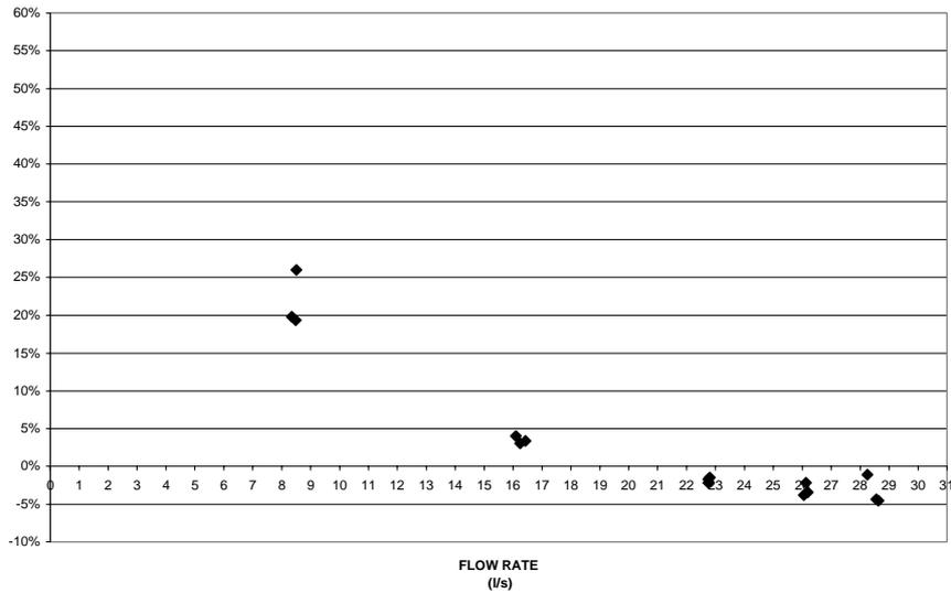
Figure 3 Electromagnetic flow meter error curve.
