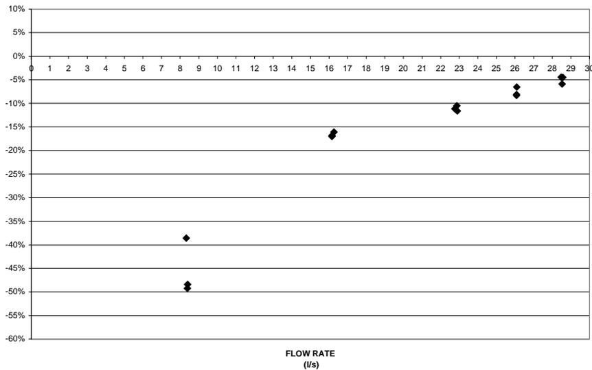
Figure 3 Ultra sonic flowmeter error curve.
