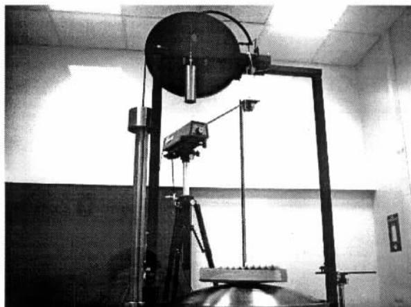
Fig.2 Setup for the calibration of the length measurement
