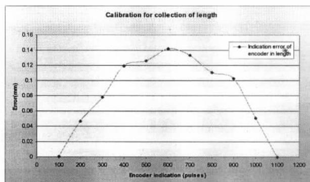
Fig.3 Error in length output from rotary encoder
