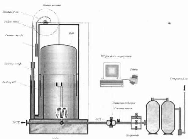
**Fig. 1** The schematic representation of the SPRING auto-bell prover gas flow standard
