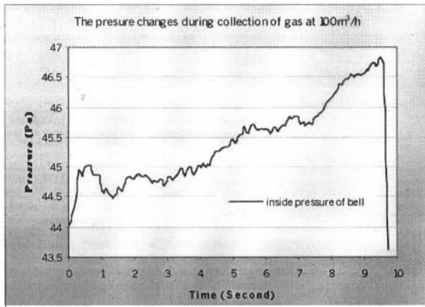
Fig.5 Pressure changes in the bell prover
