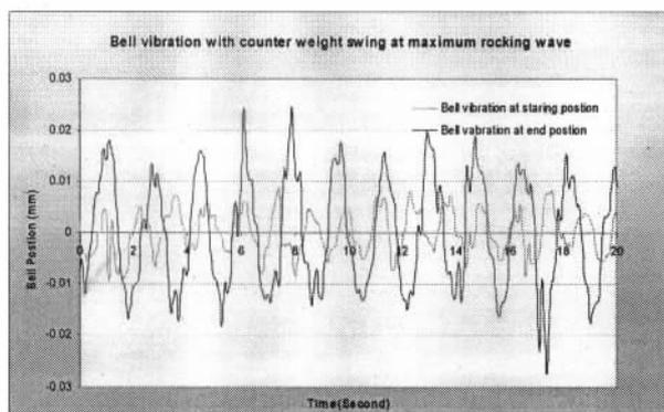
Fig.4 Bell vibration due to the counter weight swing
