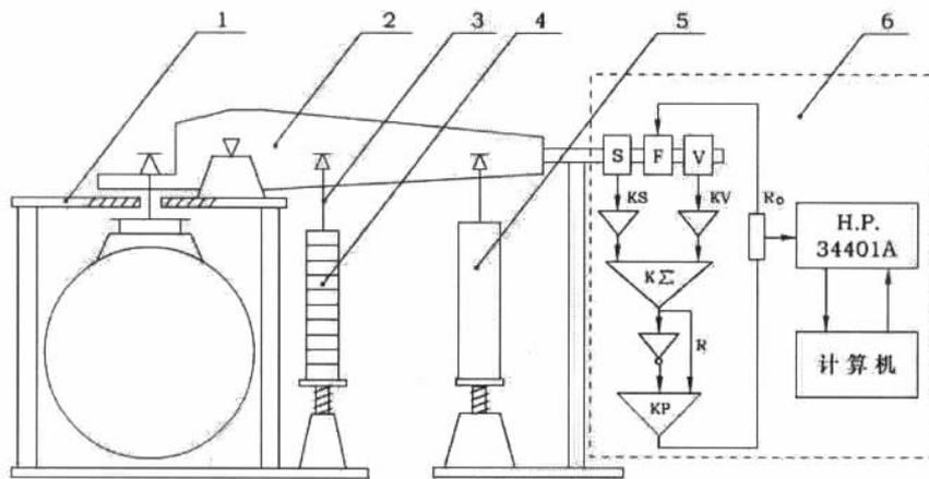
1 - supporting system      2 - beam system      3 - hanging system
