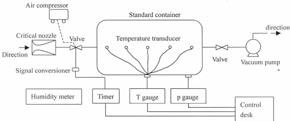
Figure 1 Structure of gas flow primary standard with pVTt method
