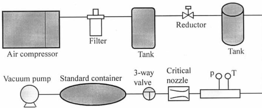
Figure 2 Structure of the facility at positive pressure
