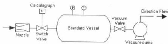
Figure 1. Schematic diagram of pVTt prover of NIM.
