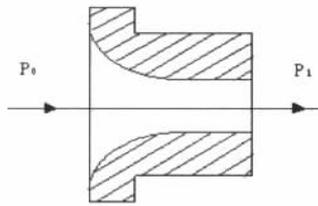
Figure 2. Schematic diagram of sonic nozzle. If the ratio of upstream gas's pressure ( $p_0$ ) and downstream gas's pressure ( $p_1$ ) are less than critical pressure ratio, then the velocity of gas flow at throat of sonic nozzle reaches sonic speed. In ideal conditions, the mass flow of gas that passes through sonic nozzle is
