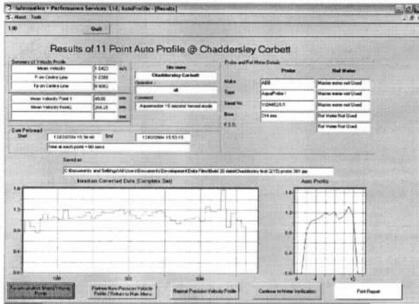
Fig 2: Profile results, probe in S2 mode
