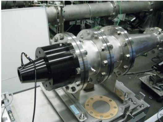
Fig. 1 Photograph of conversion nozzle unit
