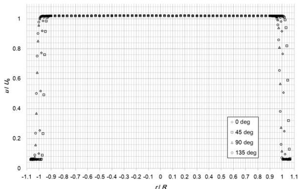
Fig.8 Non-dimensional velocity distribution (average velocity 39m/s)
