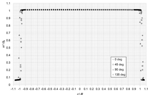
Fig.10 Non-dimensional velocity distribution (average velocity 76m/s)
