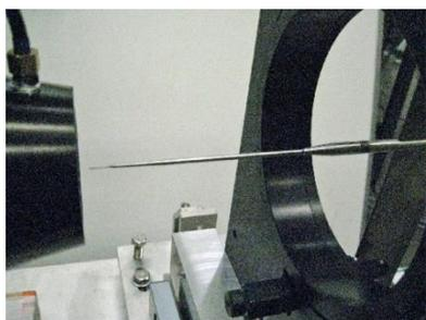
Fig. 3 Photograph of total pressure tube (measurement only total pressure)
