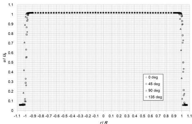
Fig.9 Non-dimensional velocity distribution (average velocity 48m/s)
