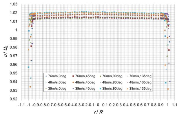
Fig.11 Non-dimensional velocity distribution (magnified and combined Figs 8~10)
