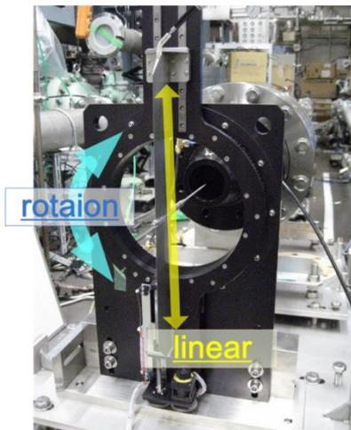
Fig. 2 Photograph of traverse device for the measurement of quantity distribution
