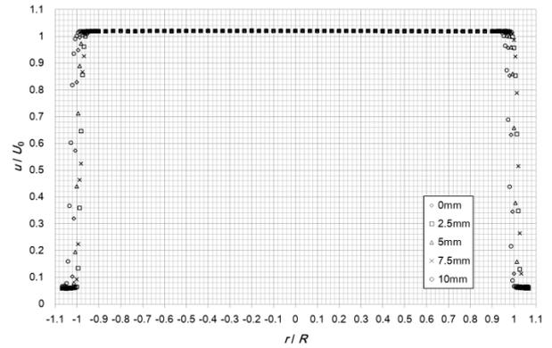
Fig. 7 Non-dimensional velocity profile at the cross-section ( $z=0, 2.5, 5, 7.5$  and  $10\text{mm}$ )
