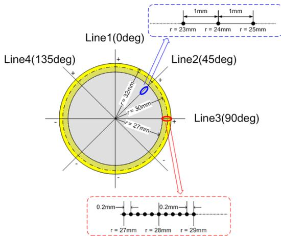
Fig. 6 Measurement point at the exit plane of the conversion nozzle
