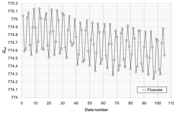
Fig. 5 Fluctuation of generated flowrate
