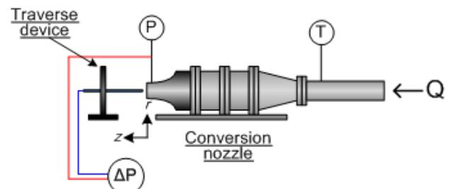
Fig.4 Experimental set-up around the conversion nozzle
