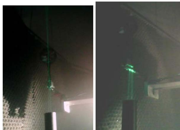
Fig 1: a) (on the left) LDA volume placement with respect to anemometer (focal length of 400,1 mm); b) (on the right) rays interrupt by the anemometer passage.
