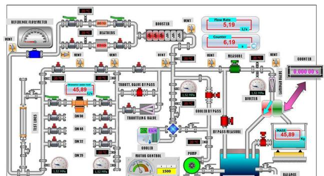
Fig. 2- Layout of scheme of the INRIM water flowrate primary standard.
