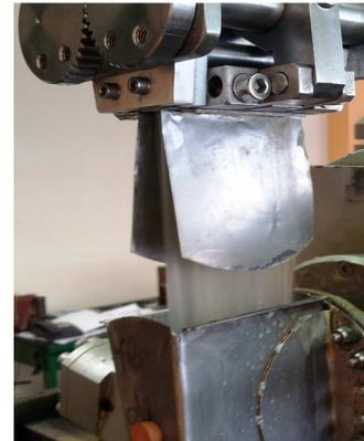
Fig. 11- Rectangular shape of water flow jet.
