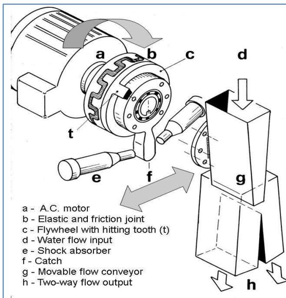
Fig 7: Scheme of INRIM diverter
