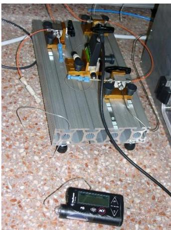
**Figure 2:** Setup of the tethered pump connected to the METAS Microflow facility.
