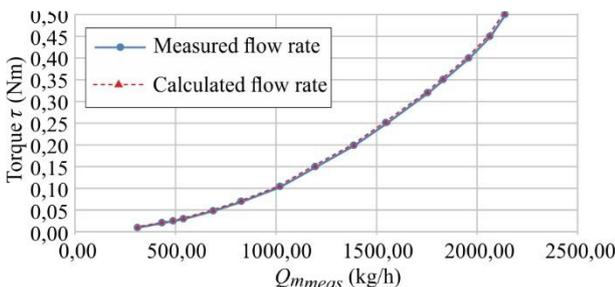
**Figure 4:** Mass flow rate of water depending on the measured torque
