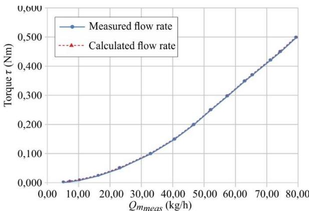
Figure 6: Mass flow rate of air depending on the measured torque
