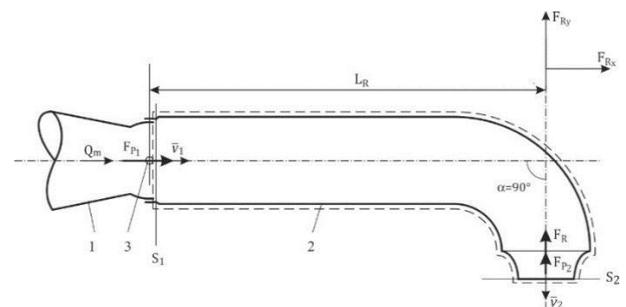
Figure 1: Configuration and the operating principle of the reaction measurement system
