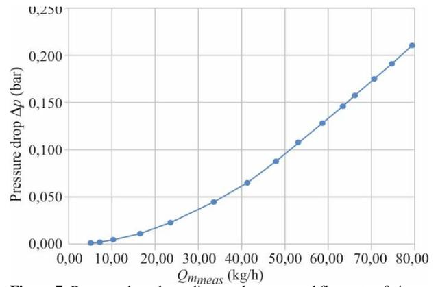
Figure 7: Pressure drop depending on the measured flow rate of air
