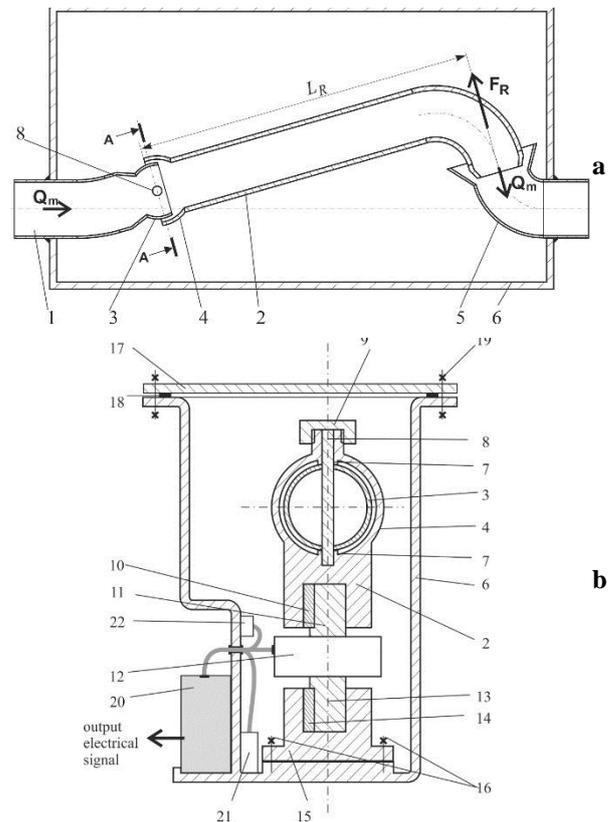
**Figure.2** Reaction flowmeter with torque measurement and horizontal collinear connections
