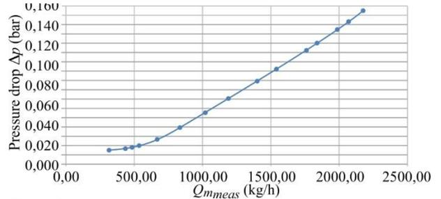
**Figure 5:** Pressure drop depending on measured flow rate of water
