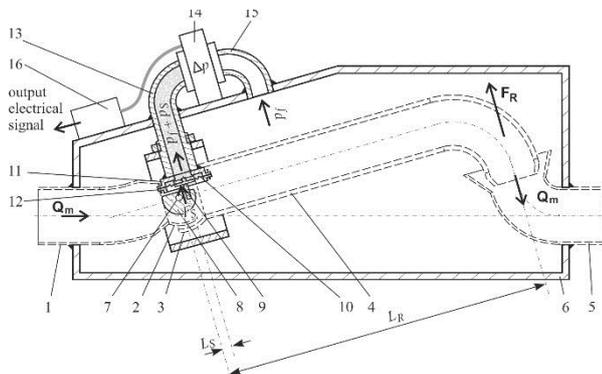
**Figure 3.** Reaction flowmeter with the measuring of the reaction force by the differential measurement of pushing (reaction) pressure.
